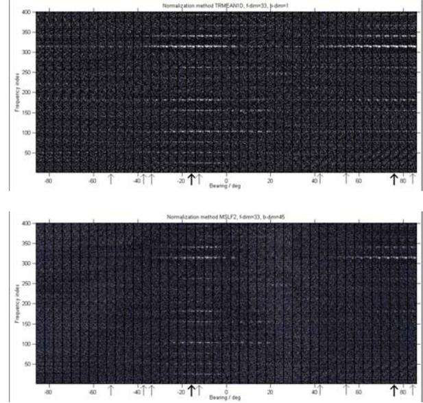
Figure 1: Multibeam LOFAR of multitarget situation, normalized by 1D-TrMean(upper fig) and MSLF2(lower fig) method
